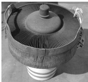
Figure 75 Example of a badly overheated tetrode. The anode fins are badly oxidized and distorted because of inadequate air flow.
